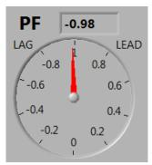
This shows the leading or laging angle and the power factor of the load.
