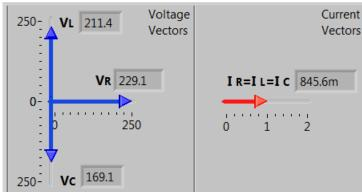
This display shows the voltage and current vectors for the selected circuit when the selection is 'vectors visible'.
