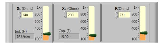
In this section you can adjust the resistor and reactance values in ohms. It displays the corresponding values of inductance and capacitance for the selected reactance.
