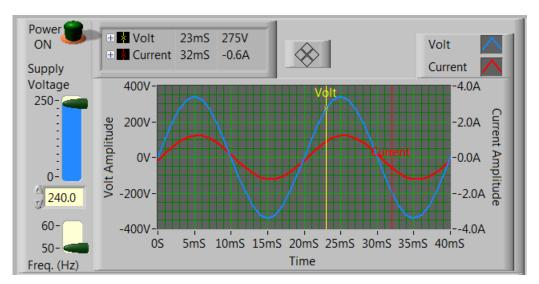
In this section you can set the supply voltage, frequency and turn on/off the power. The graph shows the voltage and current waveforms for the applied load. You can use the cursors to find the instantaneous values of voltage and current waveforms.
