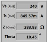
This display shows the supply voltage, supply current, load impedance and phase angle theta.
