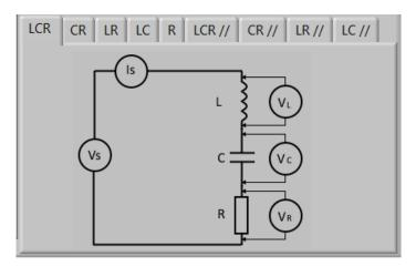
In this section you can select the type of circuit. The first five tabs select the series circuits for LCR, CR, LR, LC and R. the remaining four tabs select the parallel circuits for LCR, CR, LR and LC. When you select one tab, the corresponding circuit is displayed and it shows the meters connected to each component.
