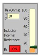
In this section you can turn off the internal resistance of an inductor (ideal case scenario) or turn on and adjust the resistance value of the inductor.
